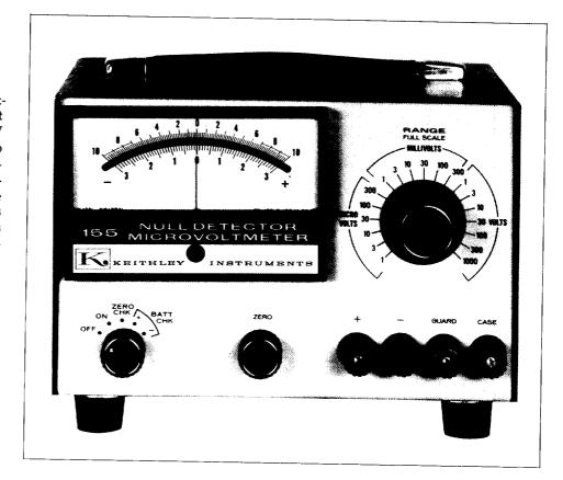
**RANGE:**  $\pm 1\mu V$  full scale to  $\pm 1000V$  on zero center meter in 19 overlapping  $1\times$  and  $3\times$  ranges.
