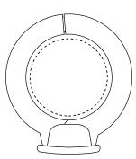
Jaw Opening: 4.4" (112mm) Conductor Size: 4.4" (112mm)
