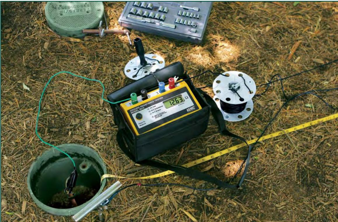
Ground Resistance Tester Model 4610 checks the ground rod using the Fall-of-Potential method.
