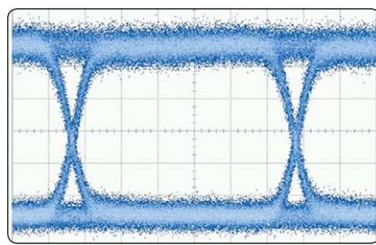
Observed jitter can be significantly reduced through a compliant clock recovery circuit
