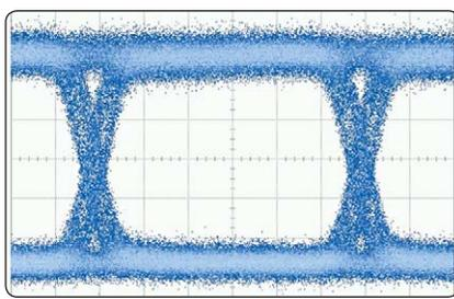
and jitter tests. If the loop bandwidth is too wide, too much high-frequency jitter is removed from the observed signal. If the loop bandwidth is too narrow, measurements can be obscured with lower frequency jitter. This jitter is usually less important since receivers easily tolerate this. Testing with an optimal loop bandwidth assures that good parts do not appear to be bad, and bad parts do not appear to be good.
