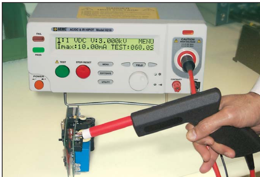
Model H215 tests a board for leakage with optional HV Test Pistol.
