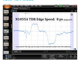
Accurate time domain reflectometry/transmission and S-Parameter measurements
